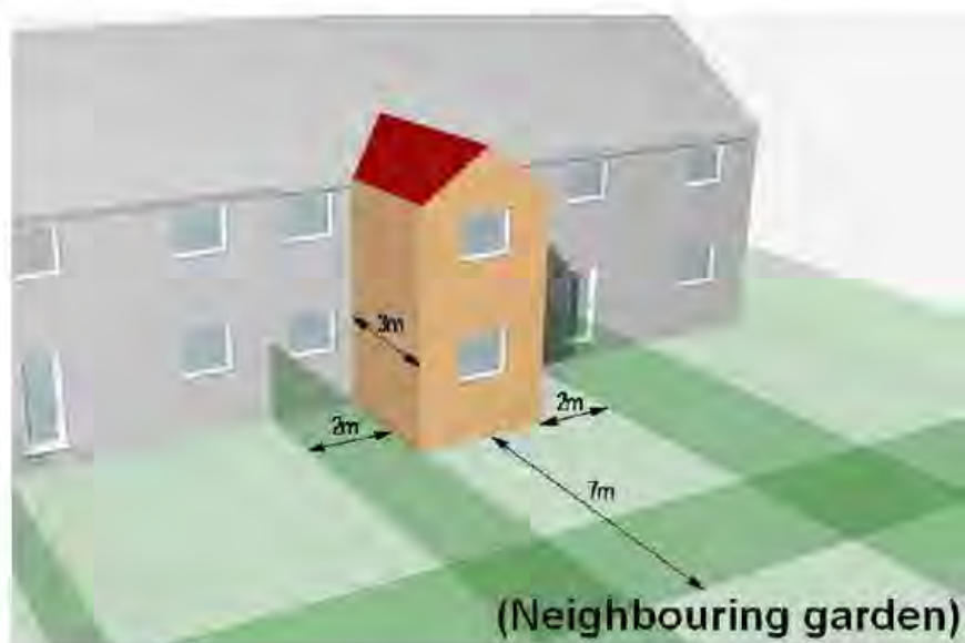
Illustration 2: Two storey rear extension to terraced house
